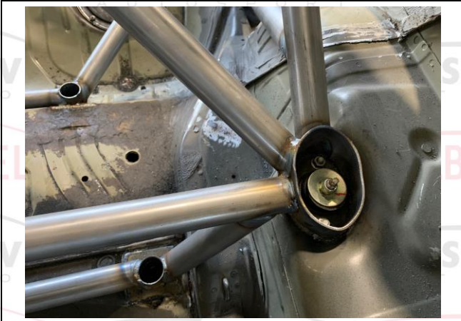
PHOTO 5 REAR BACKSTAY TO BODYSHELL ATTACHMENT
