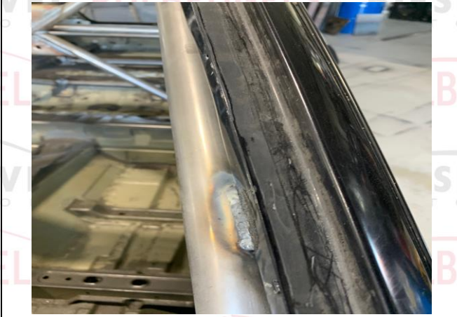
PHOTO 7 FRONT ROLLBAR TO "A" PILLAR ATTACHMENT
