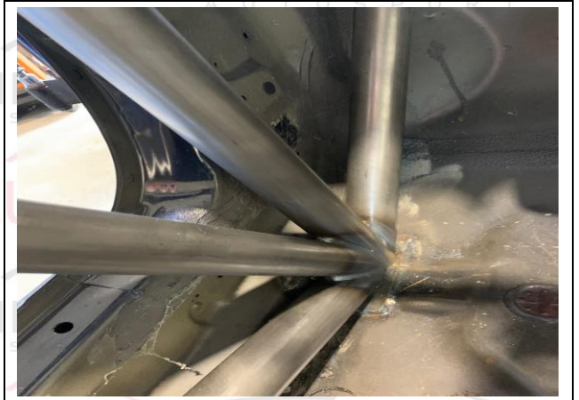
PHOTO 6 FRONT ROLLBAR TO FLOOR ATTACHMENT
