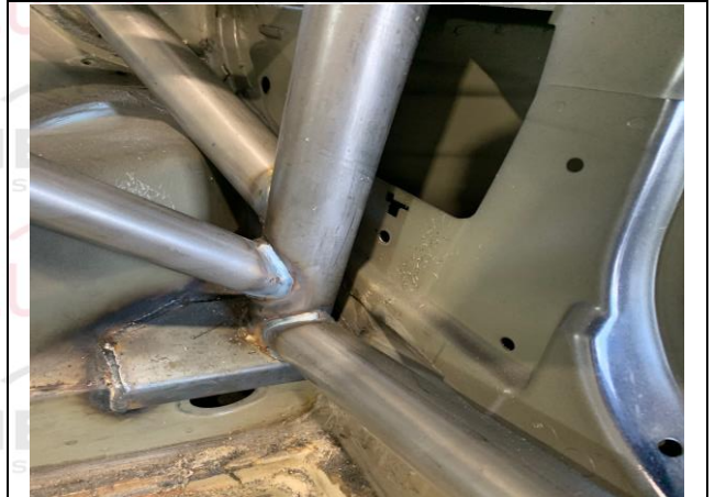
PHOTO 4 MAIN ROLLBAR TO FLOOR ATTACHMENT
